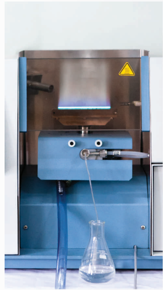
Auto Burner Assembly with Air - Acetylene Flame
