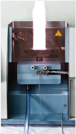
Auto Burner Assembly with Nitrous - Acetylene Flame
