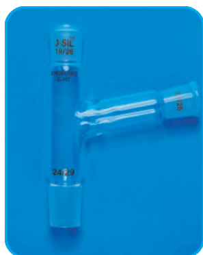
516 Adapter Multiple, Three Necks, Two Parallel and One at Angle
